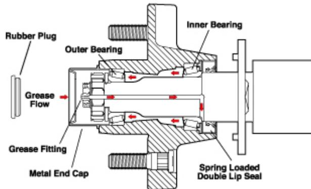
Your maintenance will stay the same as recommended by the trailer manufacturer. The big difference with using the Sport Model Bearing Protectors is that the hub is now pressurized and will not allow a vacuum to occur preventing water entry when the trailer is submerged. The reason now you would do a grease exchange is because of wear and tear over time and not to expel contaminants. The maintenance schedule can be based on a time interval or mileage interval,
